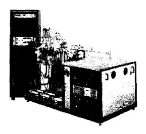
The 3D atom probe allows microscopic analysis on an atomic scale
